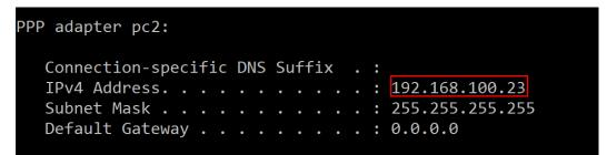
**Radar-IP: IP address form your 2<sup>nd</sup> PC** can be obtained on cmd by running "ipconfig" and check the IPv4 address of your main adapter on Radar PC
